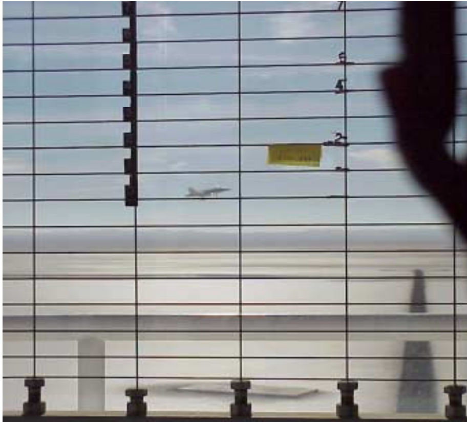
Figure 10.3 Flyby Tower Grid
