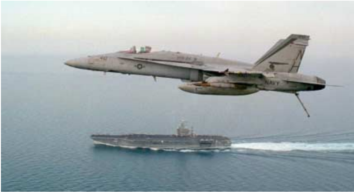
Figure 9.9 F/A-18 with Tailhook Extended
